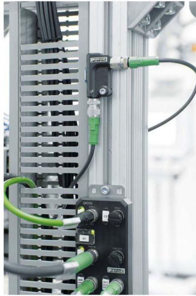
Figure 5-7 IO-Link/analog converter and Axioline E IO-Link master
